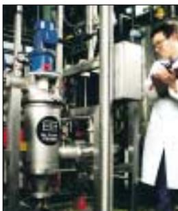
Russell Eco Self-Cleaning Filters® provide pre-filtration at a factory of H.P. Bulmer - Cider manufacturers
